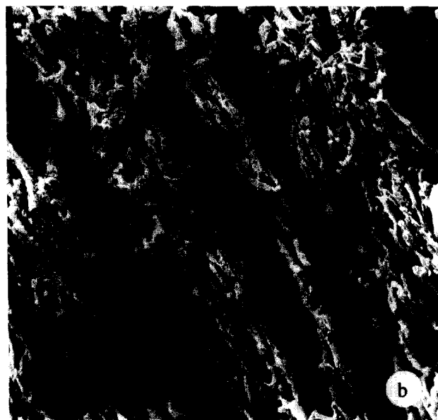
Figure 6 SEM micrographs from fracture surfaces of PIB1(W)/PE composites in ratios (a) 52.6(2.3)/45.1 (C4) that were sheared for 71 s at 1 \text{ s}^{-1} and (b) 70.8(3.1)/26.1 (C5) for 36 s. The arrows indicate the radial direction of the disc-shaped samples
